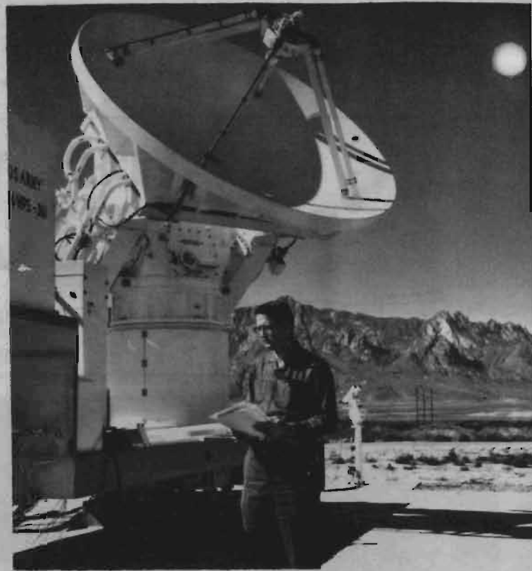
MOBILE RADAR - This is the new mobile instrumentation radar, the AN/MPS-36, developed for WSMR by the Radio Corp. of America. RCA operates the radar under an Army contract. The antenna is mounted on a 36-foot trailer. The system can be towed at speeds up to 60 miles an hour and moved from place to place on the range, and can be ready for operation eight hours after arrival at a tracking site. (U.S. ARMY PHOTO)
